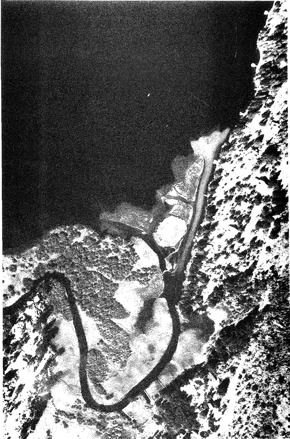
**Figure 8.** Sediment deposition at inlet to Silver Lake, Mono County, California, on October 4, 1989. Photograph courtesy of California Department of Transportation.
