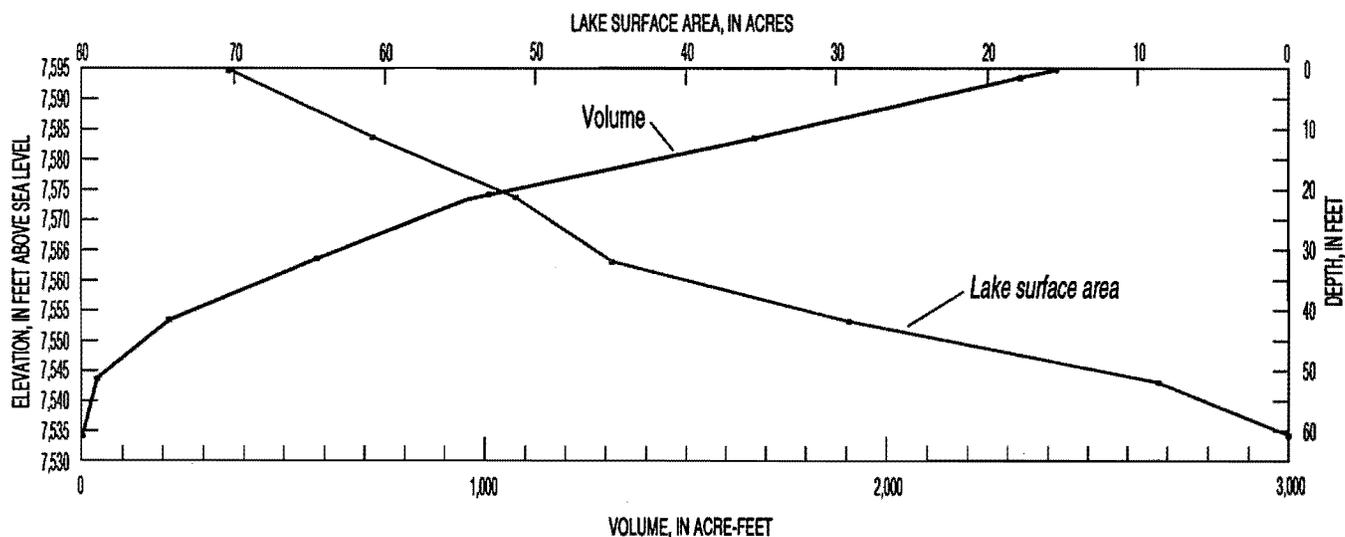
**Figure 4.** Area-volume curves for Gull Lake, Mono County, California. Date of survey September 27, 1994. All elevations based on California Department of Transportation bench mark CT 2, elevation 7,618.24 feet; center line hole punch on bolt head of fire plug at intersection of Leonard and Bruce Streets, June Lake.
