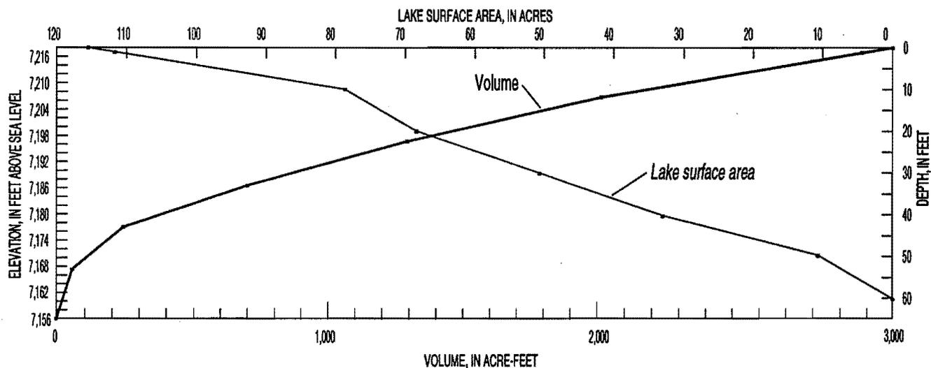
**Figure 5.** Area-volume curves for Silver Lake, Mono County, California. Date of survey September 29, 1994. All elevations based on California Department of Transportation bench mark PM 7.07, elevation 7,226.31 feet; aluminum cap on 1-in. IP, 0.3 feet below ground, 1 foot east of right edge of pavement, 14.4 feet right of centerline stripe of Highway 158, Mono County, across from entrance to Silver Lake Resort Trailer Park, 10.5 feet west of metal witness post.
