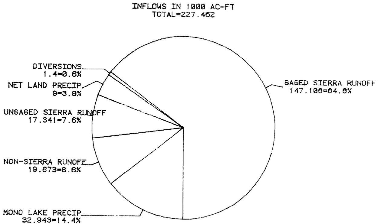
Figure 4-1 Inflows and Outflows to the Mono Groundwater Basin in 1975 Water Year
