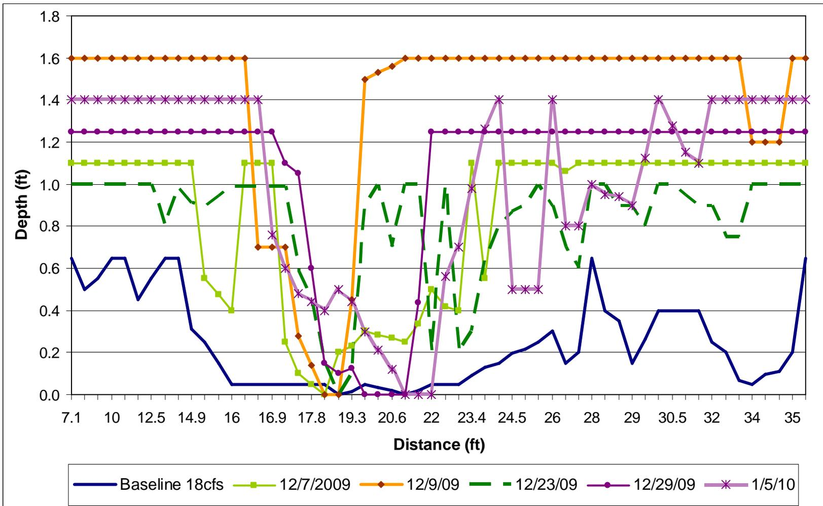
**Figure 13.** The anchor ice dams formed between Tran\_DR and Tran\_DP on December 9. The dam height reached 1.6 ft resulting in flooding and subsequent freezing over and around the dam. This was the worst anchor ice forming event during the study.
