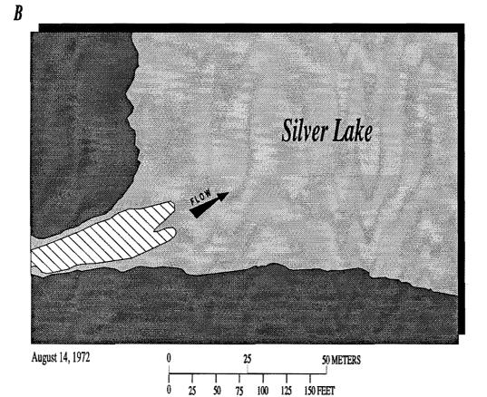
Figure 10. Location and size of sedimentation area at inlet to Silver Lake, Mono County, California.
