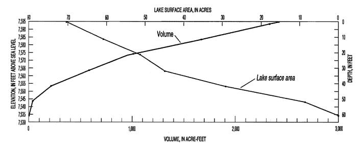
**Figure 4.** Area-volume curves for Gull Lake, Mono County, California. Date of survey September 27, 1994. All elevations based on California Department of Transportation bench mark CT 2, elevation 7,618.24 feet; center line hole punch on bolt head of fire plug at intersection of Leonard and Bruce Streets, June Lake.
