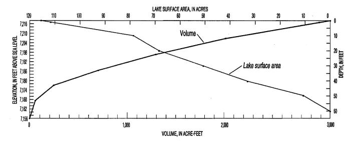
**Figure 5.** Area-volume curves for Silver Lake, Mono County, California. Date of survey September 29, 1994. All elevations based on California Department of Transportation bench mark PM 7.07, elevation 7,226.31 feet; aluminum cap on 1-in. IP, 0.3 feet below ground, 1 foot east of right edge of pavement, 14.4 feet right of centerline stripe of Highway 158, Mono County, across from entrance to Silver Lake Resort Trailer Park, 10.5 feet west of metal witness post.
