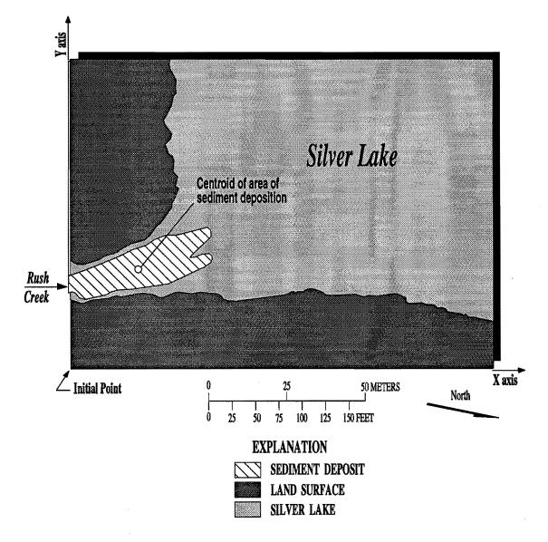
Figure 9. Centroid of typical sediment deposition at inlet to Sliver Lake, Mono County, California.
