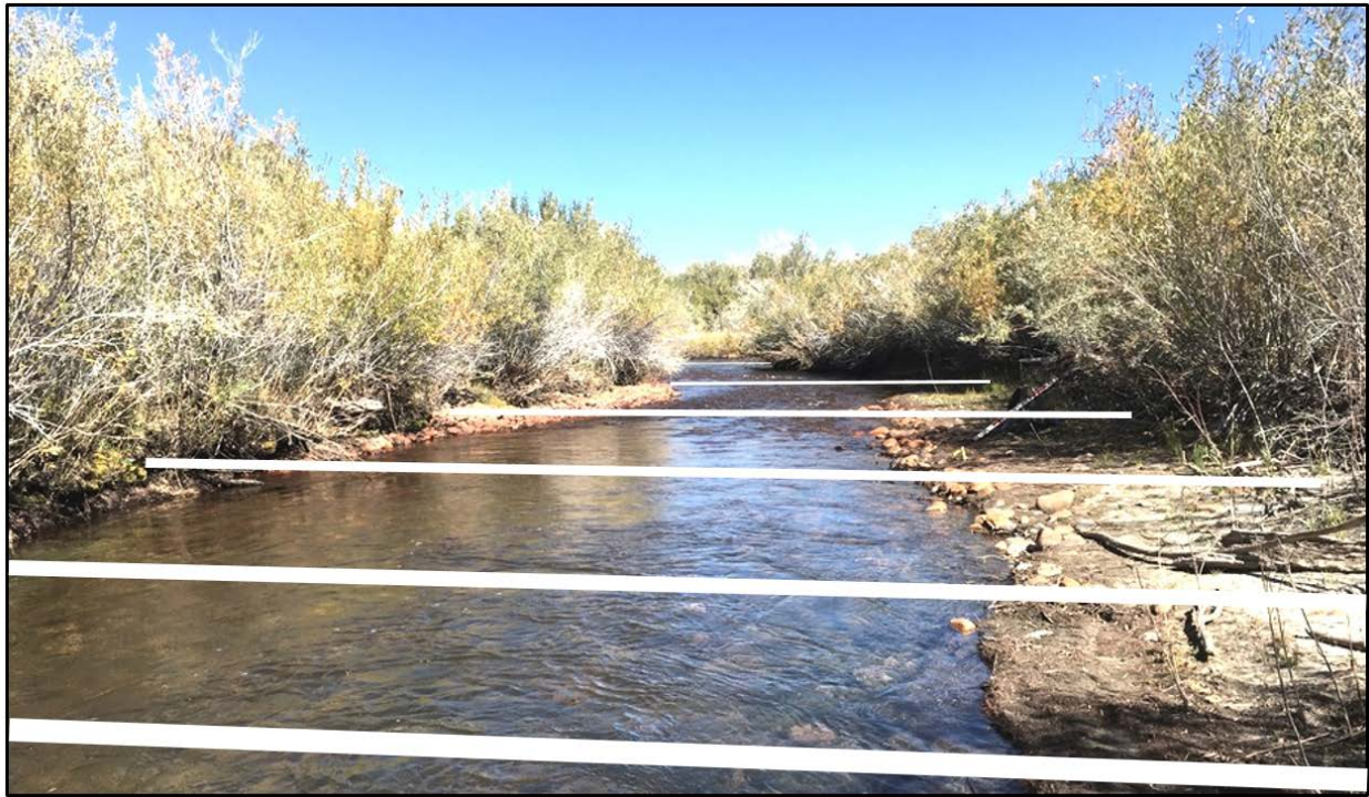
Figure 37. Active channel ( Q_{ACT} ) stage height between willow benches in Lower Rush Creek at HU No.2 (looking downstream from RCT). Streamflows exceeding Q_{ACT} trigger the onset of bankfull channel control.
