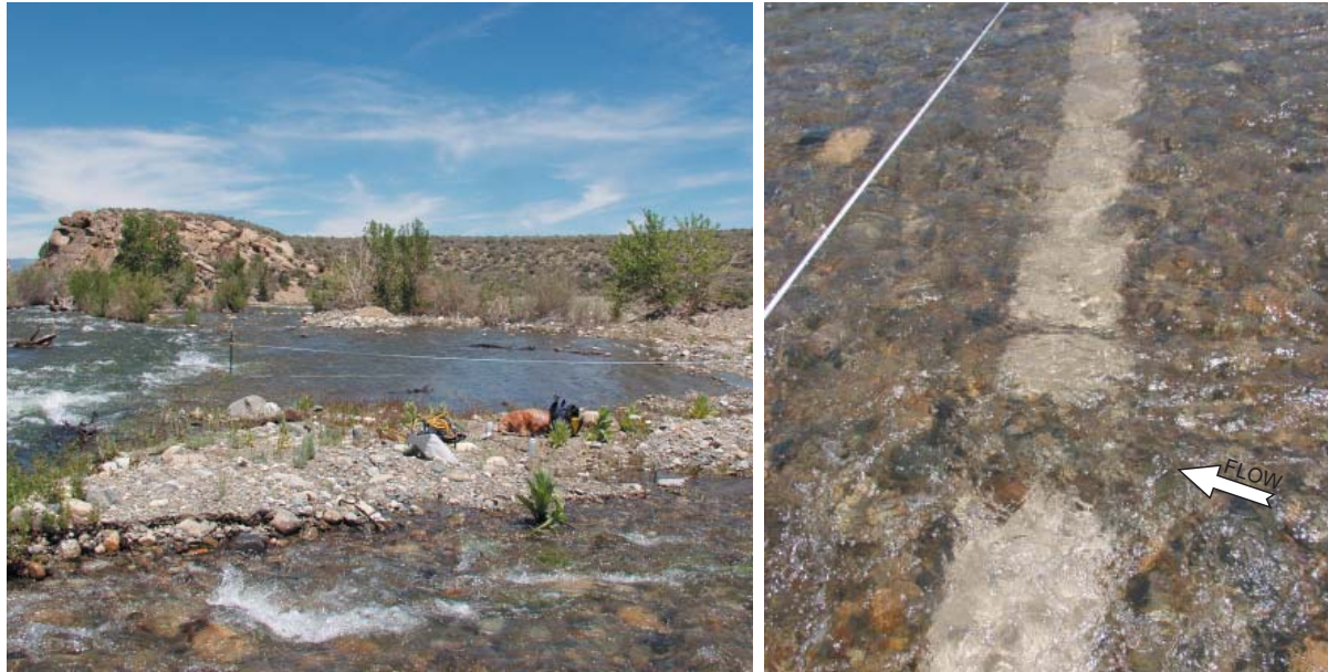
Figure 34. The 3-D constructed floodplain monitoring site on 6/11/04 (approximately 384 cfs) showing virtually clear water on passive fine sediment traps on floodplain.
